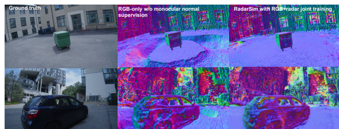
Figure 4. Normal-dependent BRDF encoding allows RadarSim to improve reconstruction of textureless regions in a joint training setting, without using monocular-predicted normals.
